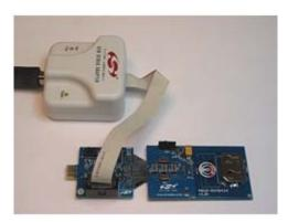
This setup is suitable for downloading, running, and debugging the program in RAM. This board has a PCB antenna and battery, so after downloading the program and starting the execution by disconnecting in the IDE, the board can be physically disconnected from the programming interface and tested in mobile form. A switch is provided on the board to connect/disconnect the battery.
